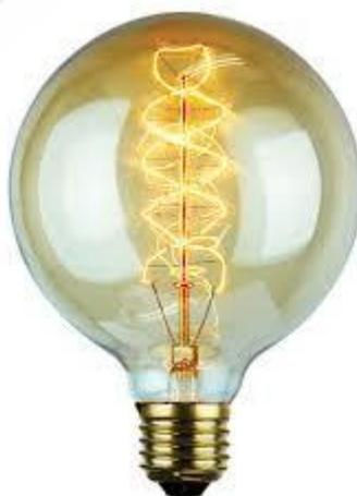
**Metal Filament Lamp** – This lamp consists of fine metallic wire either straight or coiled, which is called the filament. The filament is made up of tungsten metal and hence it is also referred to as tungsten lamp. These lamps are available in to varieties namely, vacuum type and gas filled type.
