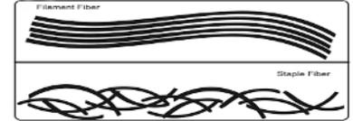
Many fibres are then twisted in Z or S shape (clockwise or anticlockwise) to form a yarn. The yarn can be two ply, three ply or more. Higher the number of ply, stronger the yarn. Also TPI (Twists per inch) of yarn is a measure of its strength and may affect its absorption qualities.
